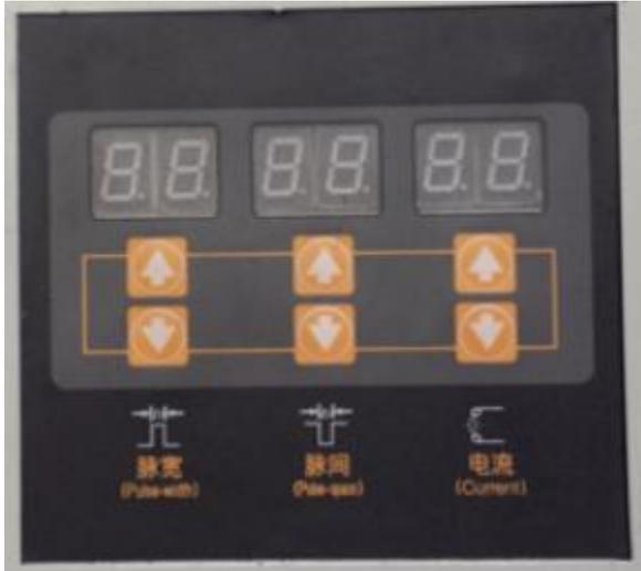
1, pulse width: The width of the spark pulse is generally set to "25" and usually does not need to be adjusted.
