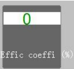
4: Standard parameters for depth. It is used to compensate the loss of the electrode piece. The larger the value, the smaller the loss, the value range is 0~100. (When the steel is scratched, it can be adjusted according to the material of the steel and the depth of the scratch). Set to 100 in the actual setting, then scratch, divide the measured actual value by the set value and multiply by 100, and then write into the efficiency coefficient.
