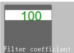
6: **Filter coefficient**: It is the short circuit time when the knife head hits the workpiece, to the set time. The knife is automatically reversed. (Usually working is to set this value to "100" in 0.01 seconds)
